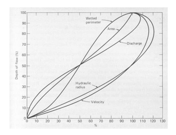
**Answer.** (a) The velocity when the pipe is full can be found from the Manning equation (SI units), noting that the hydraulic radius of a full pipe is D/4:
