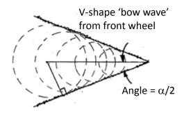
As a result, the original location of the wheel (which is also the origin of the wave), the location of the wheel after  $\Delta t$ , and the edge of the bow wave form a right triangle with the property:
