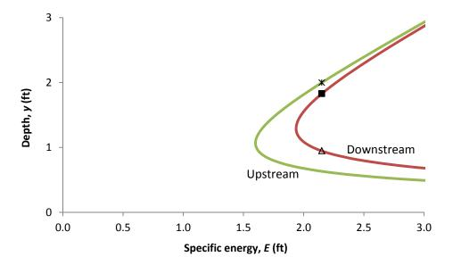
5. As in the previous problems, the specific energy diagram can be computed based simply on the value of q, which is given as 1.5 m<sup>2</sup>/s, by using the following equation:
