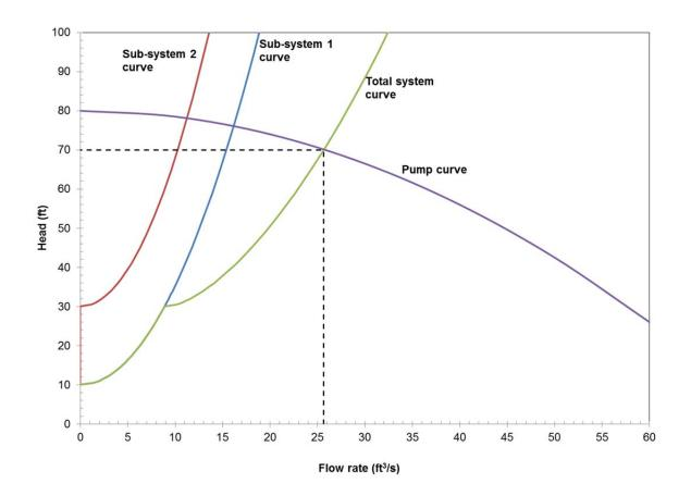
The operating point is at a flow rate of 25.7 cfs, with 70 ft of head added by the pump.
