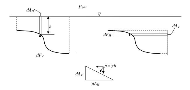
Because pressure at a given depth is the same in all directions, and because the triangle is of differential size, the pressure exerted on all three faces of the triangle is the
