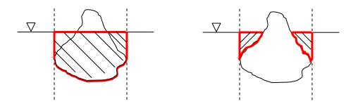
Weight of liquid in the volumes outlined in bold equals the upward force (on left) and downward force (on right) on the semi-submerged object. The difference between these two volumes equals the submerged volume of the object. Correspondingly, the net upward force equals the weight of a volume of water equal to the submerged volume of the object. Conclusion: a floating object displaces a volume of liquid that has the same weight as the object does.
