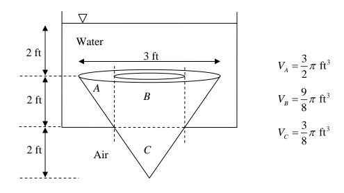
*Solution*. Section *A* of the cone is completely submerged in the water (*i.e.*, it has water both above and below it), so the buoyant force on that section equals the weight of water
