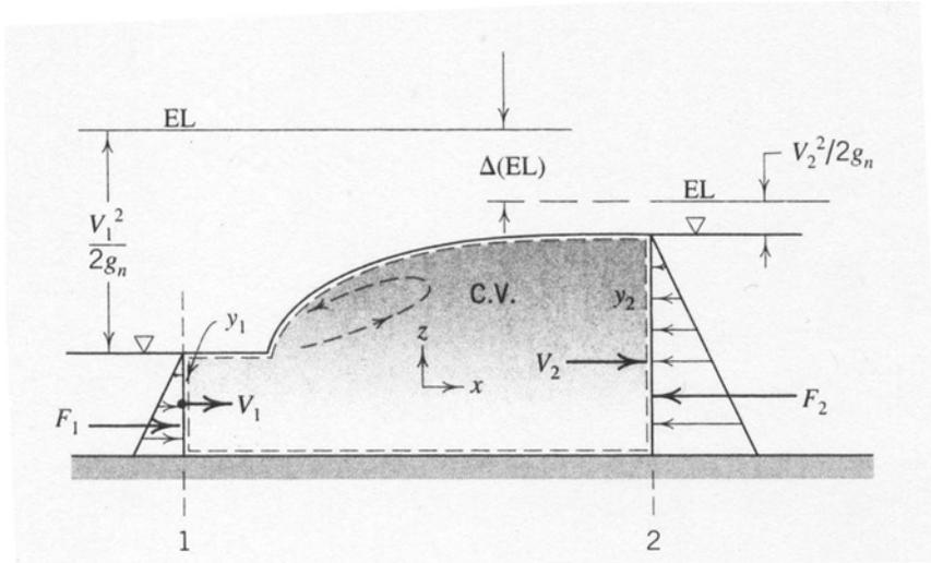
Applying the impulse-momentum equation between points 1 and 2, the only external forces acting on the fluid in the CV are the pressure-based forces on its ends, so:
