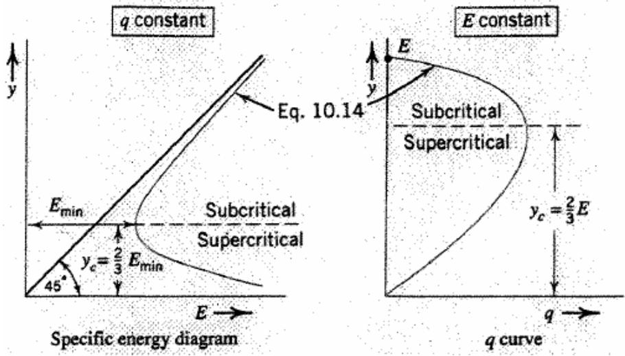
Figure 2. Plots the depth of flow as a function of (a) specific energy and (b) flow rate per unit width, in systems with open channel flow.
