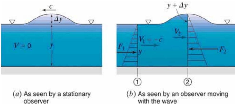
Now imagine that the water to the left (with depth  $y$ ) is caused to move with velocity  $c$  to the right. This causes the wave to become stationary relative to an observer who is outside the system and is not moving. (Note that this same scenario could be established by having the observer move with velocity  $c$  to the left, without movement of the underlying water.) As the water goes under the wave, it slows down in accord with the continuity equation, as follows.
