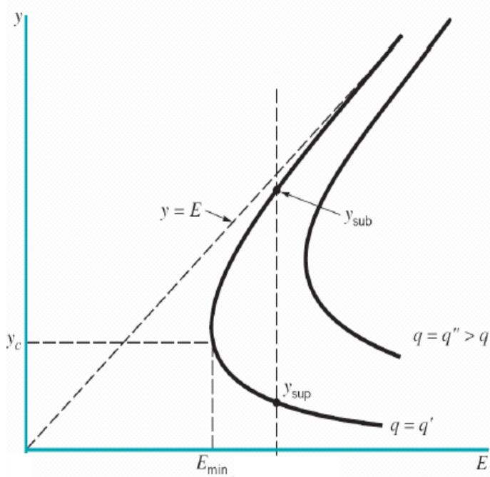
**Figure 1. A typical specific energy diagram.**
