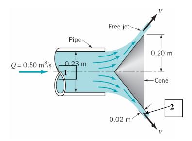
3.87. If we tentatively assume the air is incompressible (i.e., that it has constant density, an assumption we will check later), we can write Bernoulli's equation between points 1 and 2 (as shown in the diagram), as follows:
