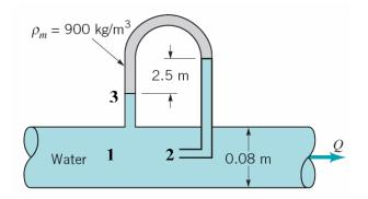
3.47. We can choose points 1 and 2 to be at the same elevation as the opening in the tube, with point 1 sufficiently upstream that the fluid is unaffected by the tube. Also, define l as the vertical distance between point 3 and either point 1 or point 2. Write the Bernoulli equation between points 1 and 2 we find:
