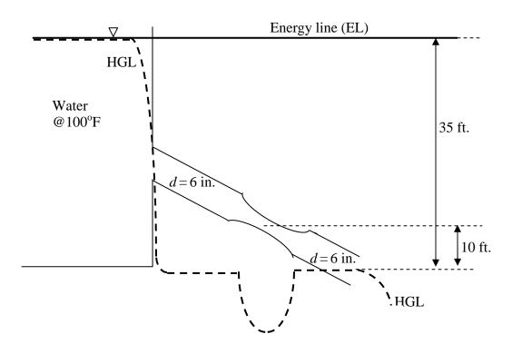
To quantify the description given above and calculate the critical diameter, we note that the density and vapor pressure of water at  $100^{\circ}$ F are given in tables at the back of the text as 62.0 lb/ft<sup>3</sup> and 0.95 psia, respectively. The pressure head of the atmosphere is:
