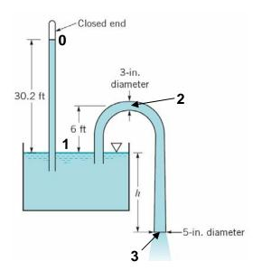
3.39. Cavitation will occur at point 2 when the pressure at that point drops below the vapor pressure of water. That pressure is present at point 0, where the velocity is zero, so if we write the Bernoulli equation between points 0 and 2 we find:
