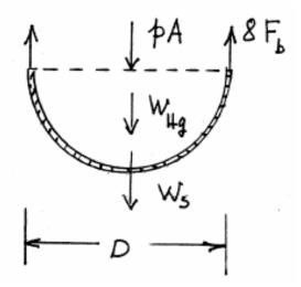
For the sphere to remain stationary, the sum of the vertical forces on the free body must equal zero. The downward forces on the body include (1) the pressure-based force on the upper surface and (2) the weight of mercury and the material forming the lower hemisphere of the container. The only upward force is that on the eight bolts. Therefore, the force balance can be written and solved as follows:
