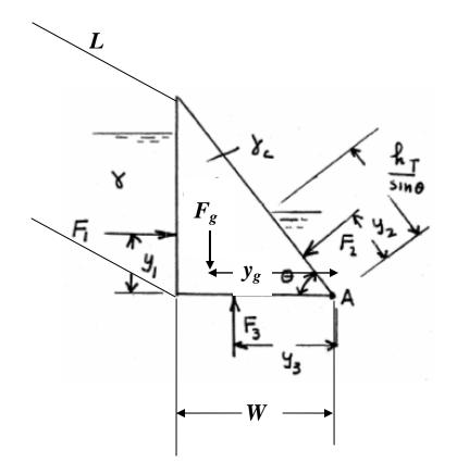
We can write expressions for  $F_1$ ,  $F_2$ ,  $F_3$ ,  $y_1$ , and  $y_2$  directly based on the system geometry and the fact that the three surfaces of interest are all planer. Specifically, we know that the pressure-based force exerted on a plane surface by a uniform fluid has magnitude  $\gamma h_c A$ , where  $h_c$  is the pressure at the centroid, and that the direction of the force is perpendicular to the plane. Thus, the forces shown in the free-body diagram can be represented as:
