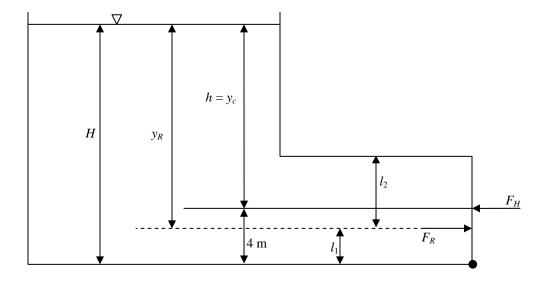
The magnitude of the resultant force exerted on the gate by the water equals the product of the pressure at the centroid and the area. Because the gate is rectangular, the centroid is at mid-depth, so the resultant force is:
