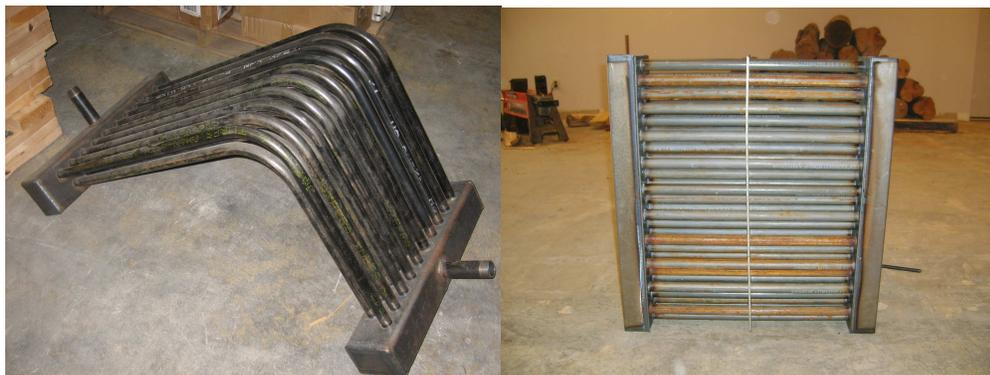
Taking into account manufacturing considerations, a tube bank of smaller  $\frac{3}{4}$ " outer diameter tubing was used, with 21 rows of 32 tubes total with an external surface area of  $1.468 \text{ m}^2$ . The original and redesigned tube banks are shown in Figure 6.3. At a reduction in materials, opening of the post-combustion path, and it is expected by conservative estimates that the increase in efficiency will maintain the desired heat output.
