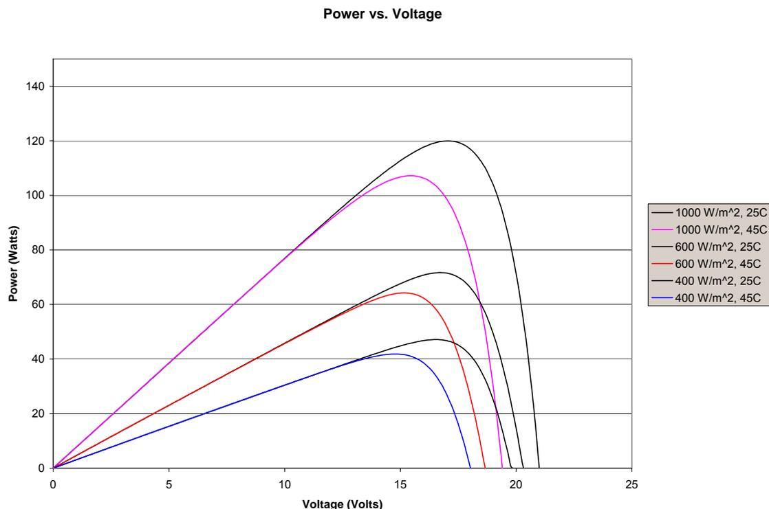
**Figure 30: Power versus voltage curves for the AP120 panels at varying incident radiation levels and temperatures<sup>88</sup>**
