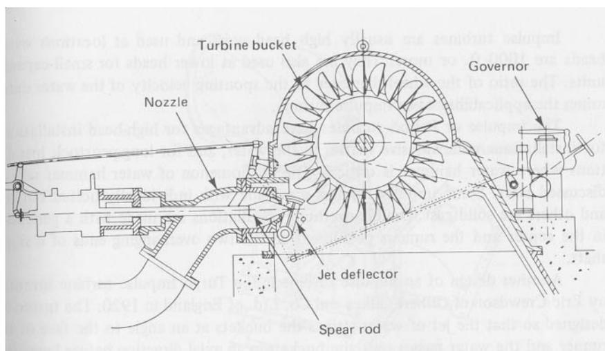
Figure 19: Pelton turbine system similar to the Stehekin system<sup>62</sup>
