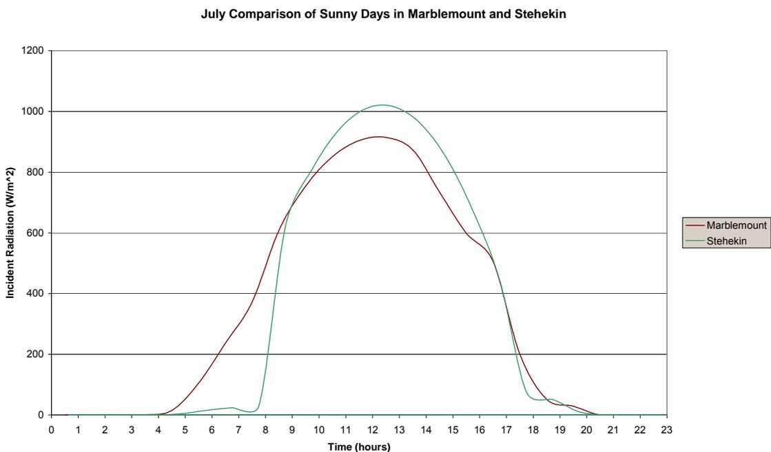
**Figure 34: July comparison of the incident radiation on a horizontal surface in Marblemount to the incident radiation hitting the panels mounted flush on the roof of the Stehekin Visitors' Center.**
