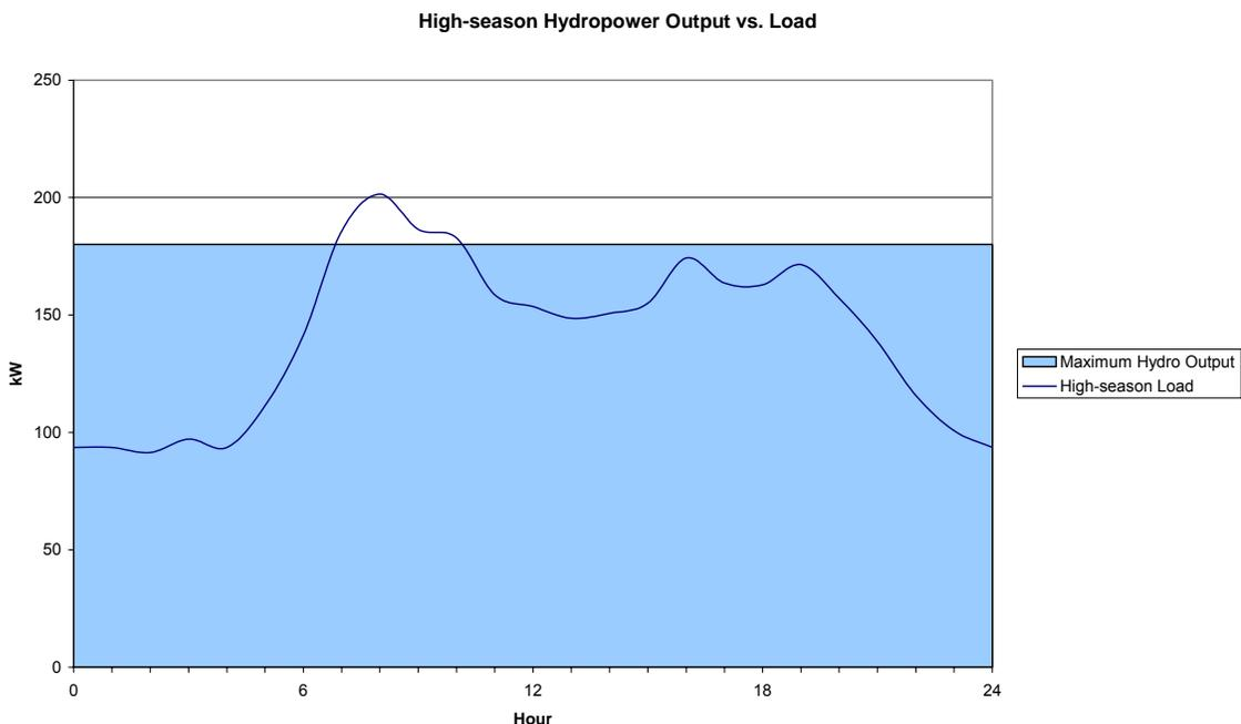
**Figure 7: Stehekin hydro output compared to electric load**
