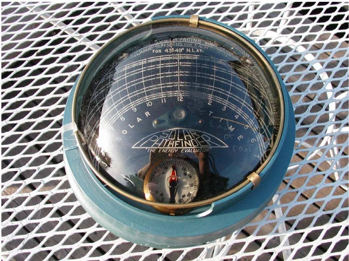
**Figure 42: The Solar Pathfinder. Notice the reflections on the left and right side of the chart that would block the sun in the morning and evening.<sup>96</sup>**
