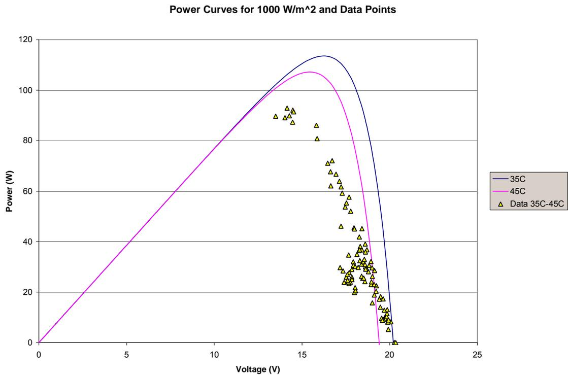
**Figure 39: Collected data points from PV array compared to the manufacturer's estimated power curves<sup>94</sup>**
