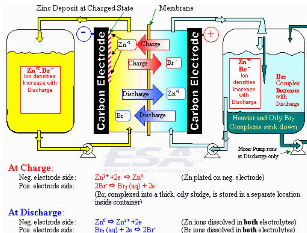
**Figure 17: The inner workings of a flow battery<sup>54</sup>**
