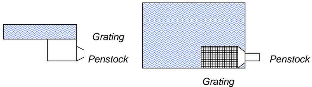
**Figure 4: Photos and diagrams of the penstock entrance on Company Creek. Photos taken in September 2003. A: Side-view of the entrance. B: Top-view of the entrance**
