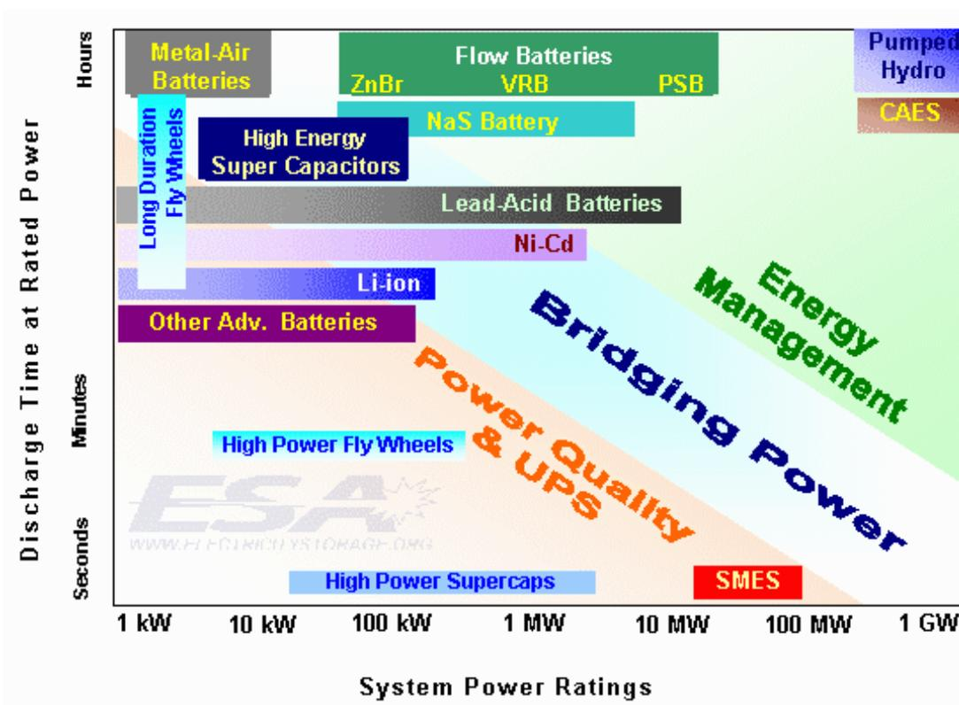
Figure 14: Discharge times and powers of energy storage technologies<sup>50</sup>
