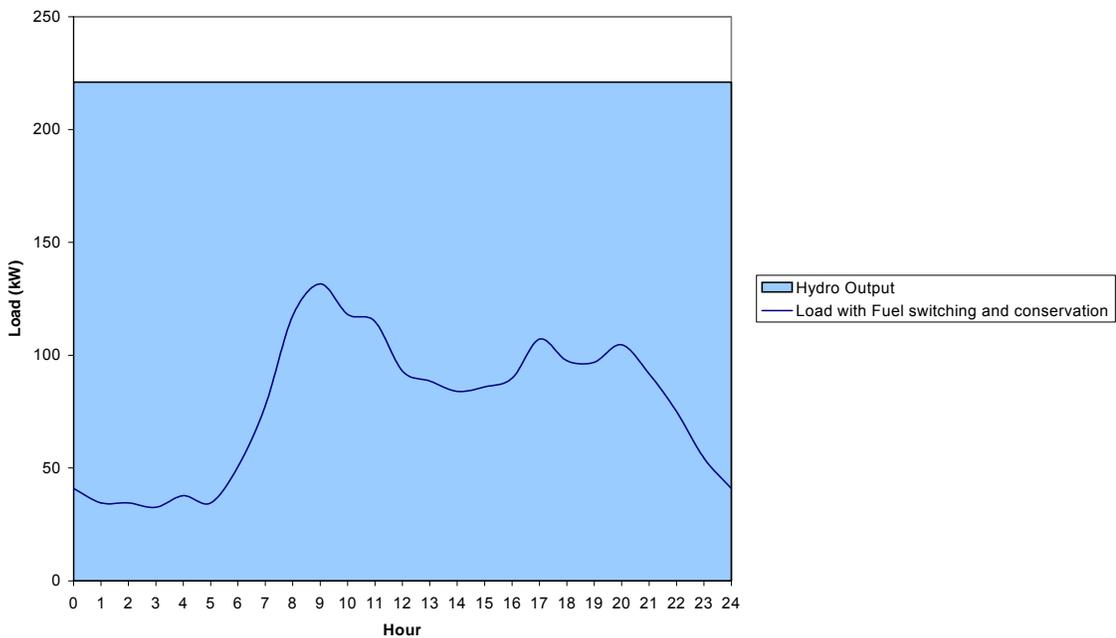
Figure 20: Reduced high-season load relative to increased hydroelectric output
