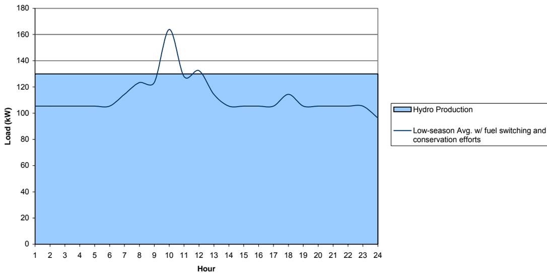
Figure 21: Reduced February load relative to increased hydroelectric output
