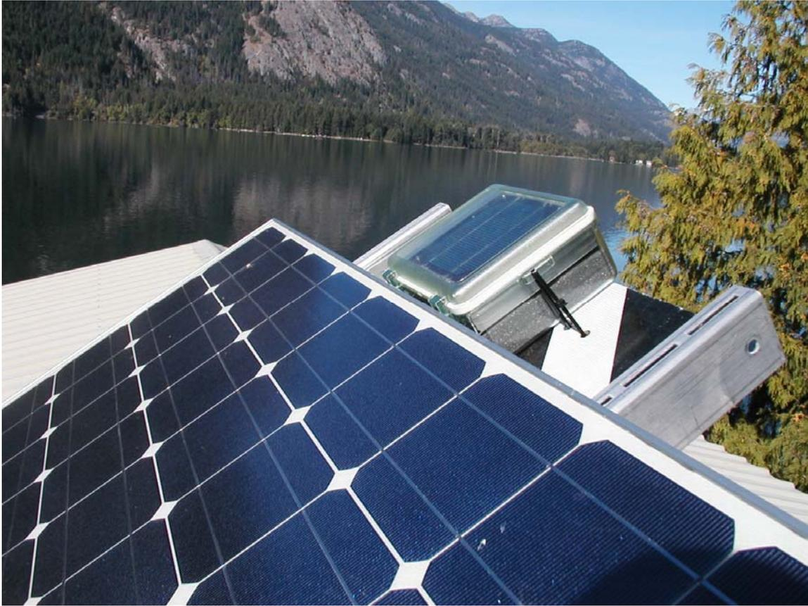
**Figure 33: Placement of the reference cell in relation to the PV panels**
