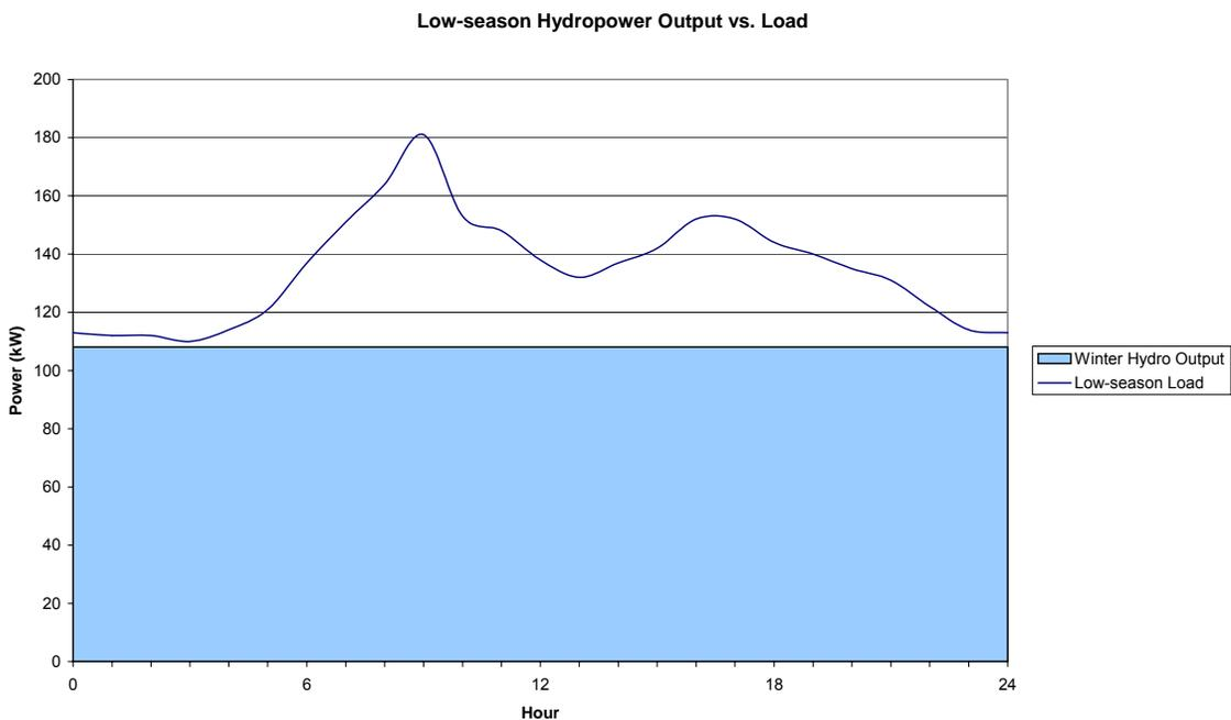
**Figure 8: Comparison of winter hydro output and electric load**
