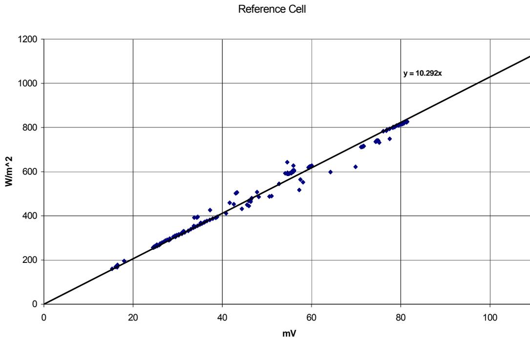
**Figure 32: The diamonds represent data points taken from the reference cell at varying incident radiation. A trend-line was then used to extrapolate to other levels of incident radiation.**
