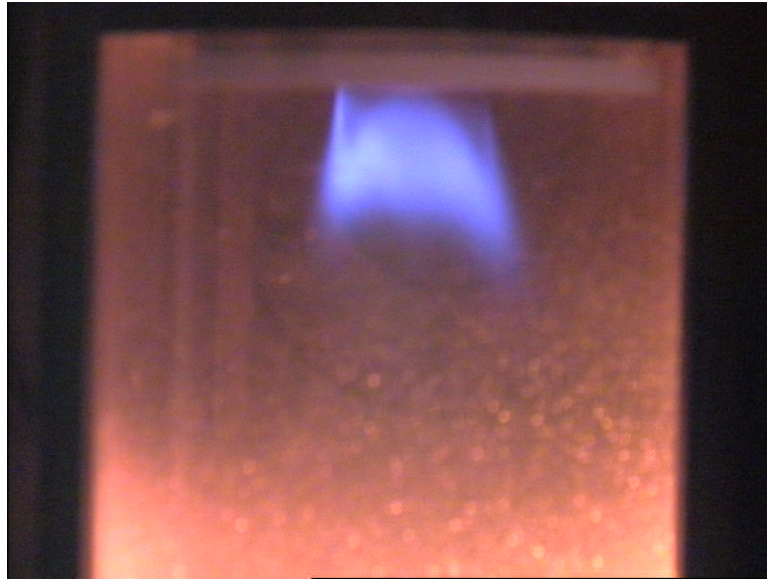
Figure 4.10: Photo of flame with a blend of 90% hydrogen and 10% methane as fuel, taken during the experiments.
