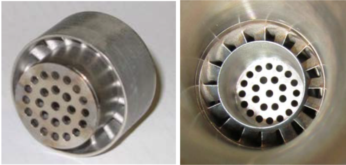
Figure 2.3: Low Swirl Injector. Right side inlet, left side outlet. [3]
