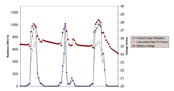
August Incident Radiation, Power Output, and Battery Voltage
