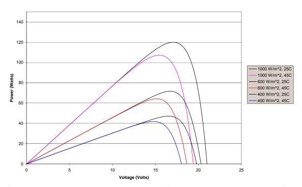
Figure 30: Power versus voltage curves for the AP120 panels at varying incident radiation levels and temperatures<sup>88</sup>
