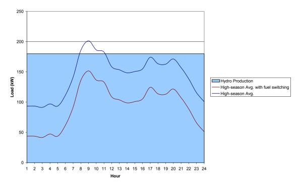
Effect, from April to October, of switching primary space heating and water heating to LPG
