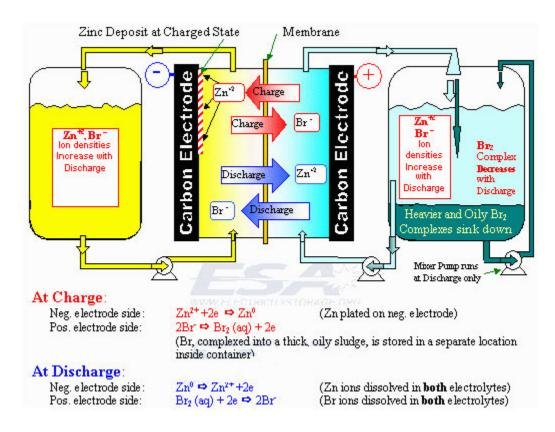
Figure 17: The inner workings of a flow battery<sup>54</sup>
