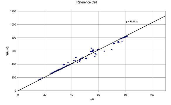
Figure 32: The diamonds represent data points taken from the reference cell at varying incident radiation. A trend-line was then used to extrapolate to other levels of incident radiation.
