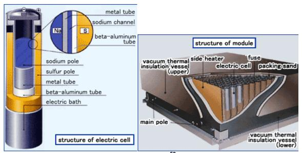
Figure 18: Diagram of NaS cell and module<sup>59</sup>
