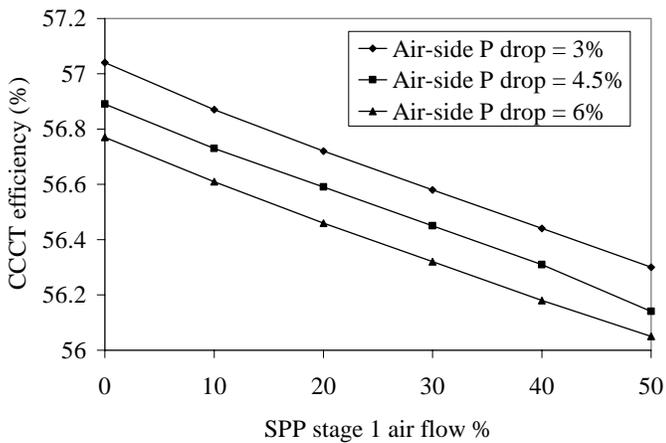
Figure 7: Variation of combined cycle efficiency with changes in air  $\Delta P$ , reheat engine. Stage 1 T = 473°C (883°F).
