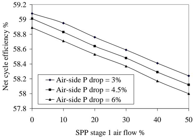
Figure 5: Variation of combined cycle efficiency with changes in air  $\Delta P$ , Frame H engine. Stage 1 T = 405°C (762°F).
