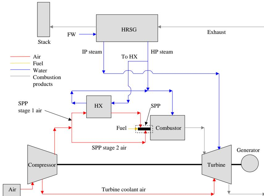
Figure 3: STIG system schematic.
