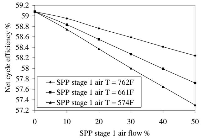
Figure 4: Variation of combined cycle efficiency with stage 1 air flow %, Frame H engine. Air  $\Delta P = 3\%$ .
