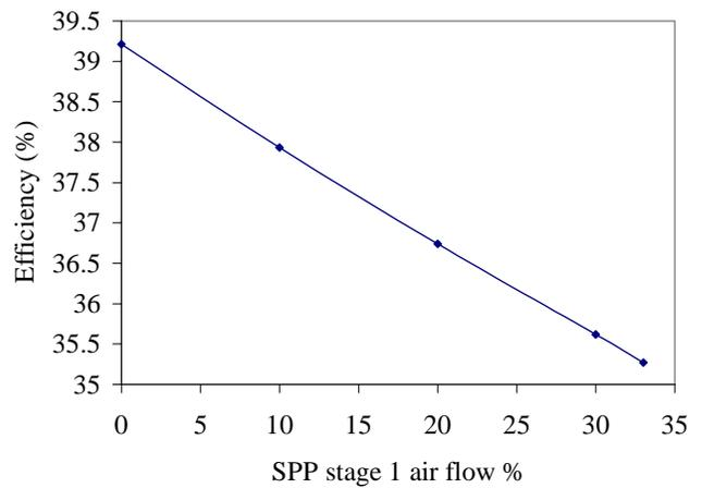
Figure 10: Variation of recuperated cycle efficiency with increasing SPP stage 1 air flow rate.
