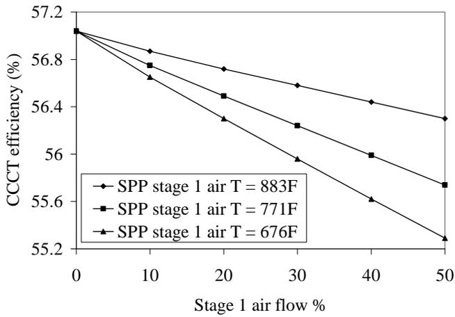
Figure 6: Variation of combined cycle efficiency with stage 1 air flow %, reheat engine. Air  $\Delta P$  = 3%.
