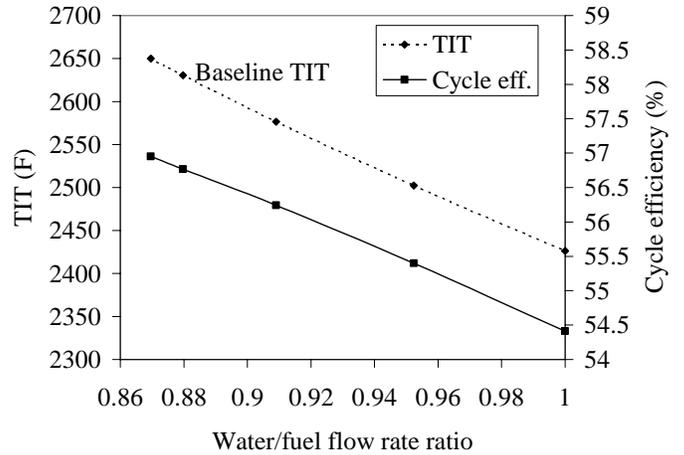
Figure 8: Variation of combined cycle efficiency and TIT with water/fuel flow rate ratio, Frame H engine.
