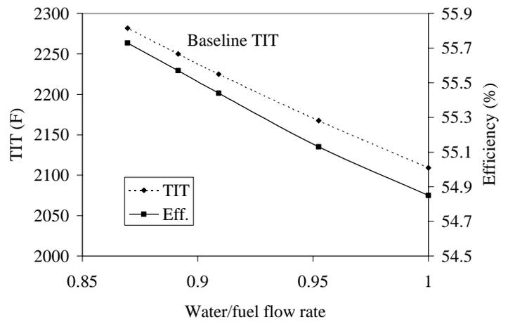
Figure 9: Variation of combined cycle efficiency and TIT with water/fuel flow rate ratio, reheat engine.
