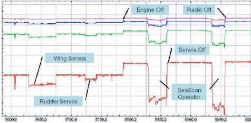
Figure 3.2: Self induced magnetic field effects. Courtesy of Boeing/Insitu.
