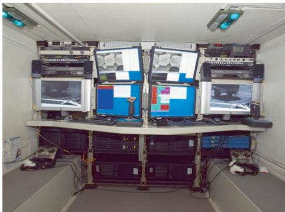
(a) ScanEagle pilot and sensor operator interface
