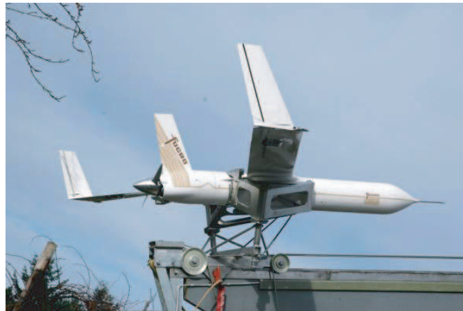
Figure 1. Image of the Fugro autonomous aeromagnetic survey vehicle, the ‘Georanger I’ by the Insitu Group.
