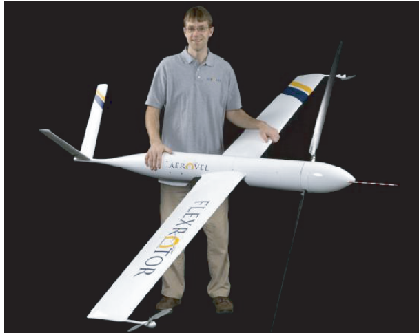
(a) Flexrotor is a unique aircraft developed by AeroVel which is able to operate in both traditional wing-borne flight and hover in thrust-borne flight.
