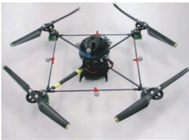
Fig. 5. Quadrotor vehicle equipped with reference markers.
