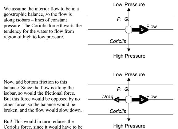
proportional to the speed of the flow. So the pressure gradient would outbalance the Coriolis force, and there would be acceleration towards the low pressure region. The flow would acquire a component down the pressure gradient.
