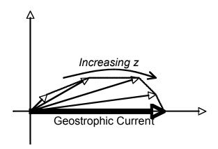
It is possible to integrate this solution in the vertical to obtain the transport in the bottom Ekman layer. The down-gradient component amounts to be  $u(A_z/2f)^{1/2}$ .
