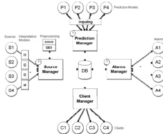
**Figure 1. The modular architecture of AEGIS ensures flexibility, scalability and robustness.**
