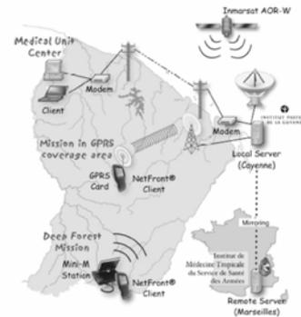
Figure 1 – Deployment schema of the military surveillance system in French Guiana
