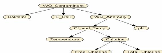
Figure 1 – Example of nodes for the Water Quality BBN.
