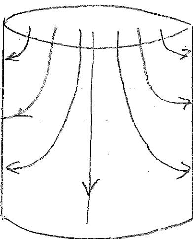
EXAMPLE: POINT CHARGE AT THE CENTER OF A GROUNDED CYLINDER.
