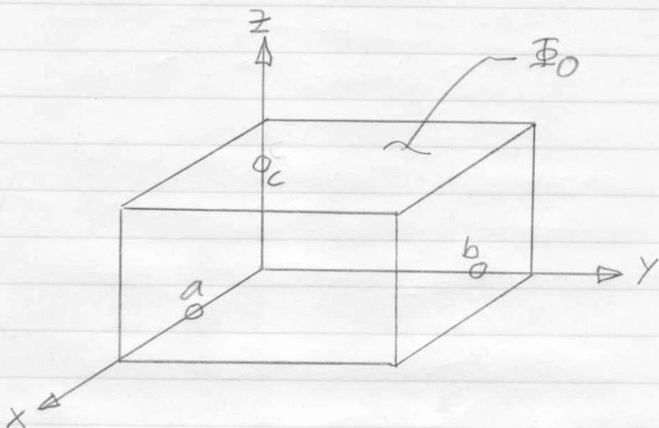
THE RECTANGULAR SURFACE AT  $z=c$  HAS POTENTIAL  $\Phi_0$ , OTHER SURFACES HAVE POTENTIAL ZERO.
