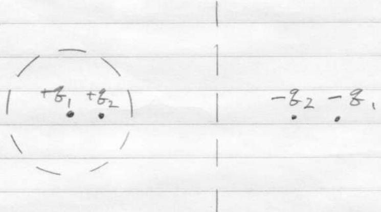
THE MAGNITUDE AND POSITIONS OF THE CHARGES ARE KNOWN FROM THE SIMPLER CHARGE-ABOVE-PLANE AND CHARGE-IN-SPHERE IMAGE CHARGE PROBLEMS:
