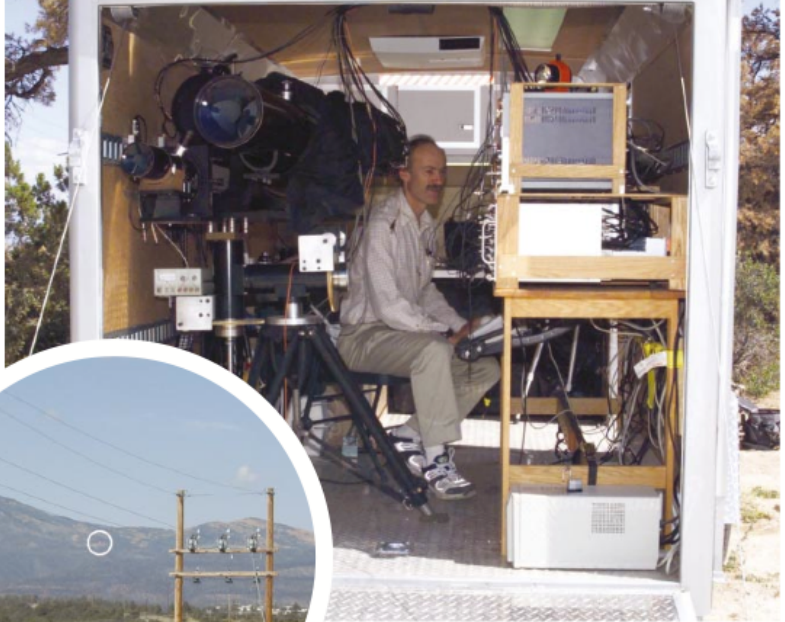
In the air: Richard Hughes has sent a photon-encrypted code from a laser source (circled, inset) to a receiver.
