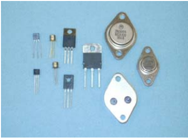
Figure 1 - Types of transistors. The left hand lower one is the one in the lab kit. The large square ones and the large metal cans are power transistors. An NPN transistor circuit symbol, with Collector, Base and Emitter marked C, B and E respectively, is on the right side of the figure.
