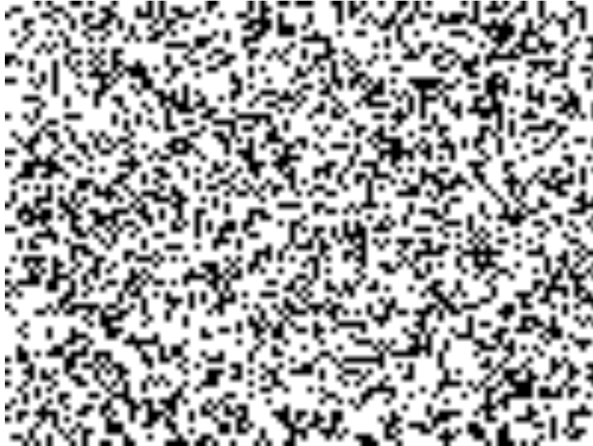
Figure 203: Typical realization of a random sampling of the image with 2500 random pixel points (black). The white pixels, which comprise 2/3 of the pixels, are not sampled. It should be noted that for images, the sampling mask can be extremely important in the image reconstruction [54].
