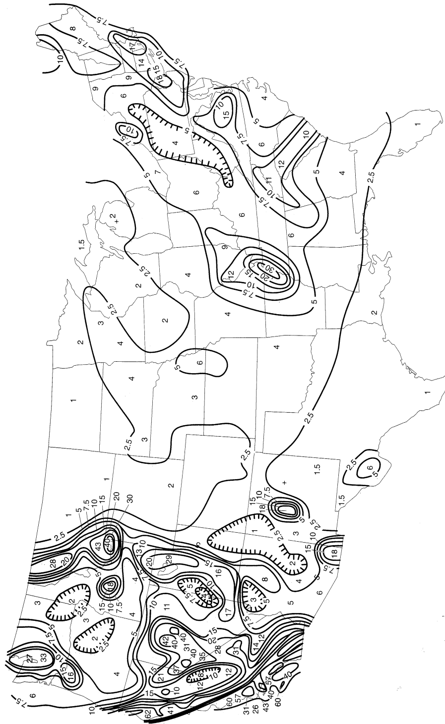
Figure 4.16 Contours of mean horizontal acceleration on rock (expressed as a percentage of gravity) with 10% probability of exceedance in 50 years. (After Algermissen et al., 1990.)
