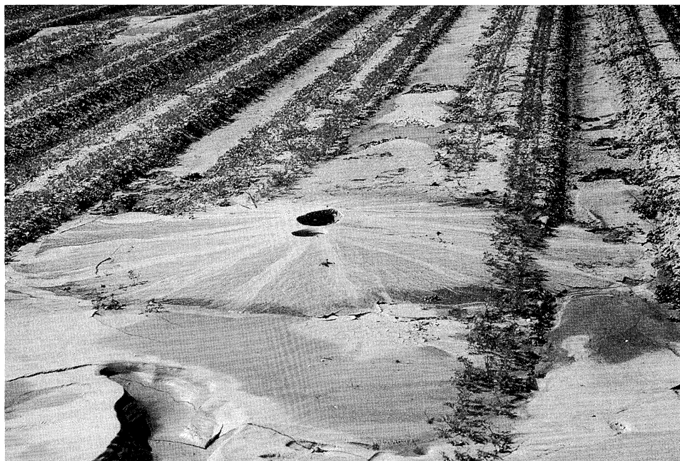
Figure 1.10 Sand boil in rice field following the 1964 Niigata earthquake (K. Steinbrugge collection; courtesy of EERC, Univ. of California).
