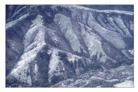
Figure 4. Aerial oblique view of Mill Creek showing debris flows in almost every tributary canyon. Debris flows extend the entire length of all of the tributary canyons to the intersection with Mill Creek.
