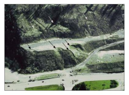
Figure 17. Numerous slumps (arrows) near Chehalis, Washington, reactivated by February storm.
