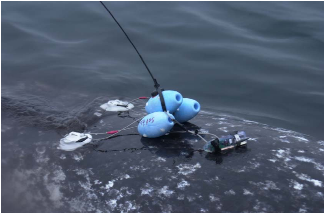
Figure 2.2. Image of suction-cup attached TDR on a narwhal in Creswell Bay, August 2000. Note the round buoys attached to the suction cup with wire. The TDR is attached underneath the buoy cluster and rests on the whale's back.
