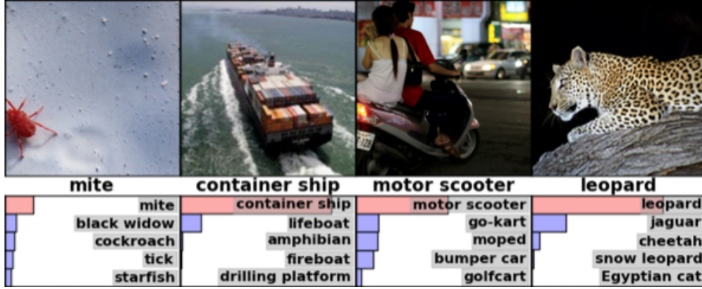
Figure 3: Object Recognition using a CNN trained with ImageNet data (from Krizhevsky, Sutskever, and G. E. Hinton 2012 )
