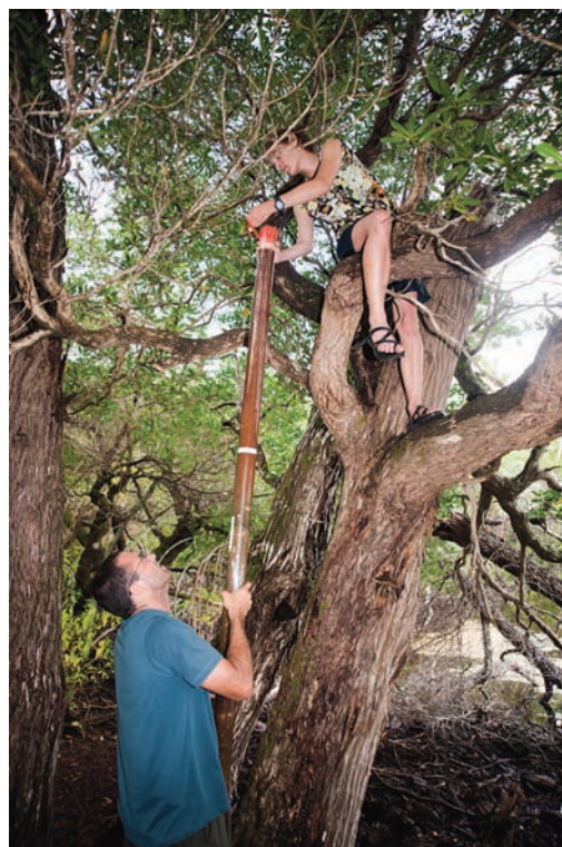
A sediment core pulled from a lake bottom on Lib Island holds preserved algae that reveal past rainfall. Trees prove handy for keeping a core vertical as thin sections are cut for the lab.
