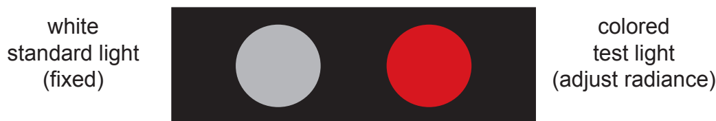
Figure 3.1: Heterochromatic brightness matching. The experimenter sets the radiance of the white standard light (appears grey in the context of this figure), and sets the colored test light to each of a series of different wavelengths in turn (appears red in this example). The subject’s task is to vary the radiance of the colored test light, to match its perceived brightness to the fixed white standard.
