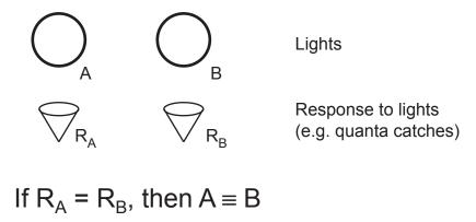
Figure 2.8: Scotopic metamers. A and B are lights of two different spectral compositions and intensities. If the intensities of A and B can be adjusted to make the two stimuli indiscriminable, A and B are called metamers. In the funnel analogy, lights A and B are indiscriminable because they make equal counts,  $R_A$  and  $R_B$ , on the counter.
