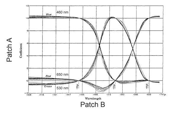
Figure 7.4: Data from a trichromatic color mixture experiment. The abscissa shows the wavelength of light in patch B. The ordinate shows the proportions of 460, 530, and 650 nm lights in Patch A required to make the two patches metameric. The lines show fits to the data from 10 subjects. The negative coefficients of the primaries in for some wavelength regions imply that the primary was moved from Patch A to Patch B. [From Wright (1928, Fig. 2, p. 148).]
