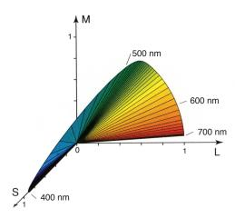
Figure 11.5: LMS cone space, with the rays for the different wavelengths shown in their typical perceived colors. The curved surface enclosed by all the rays is called the spectrum locus. The "purple" line connects the two ends of the spectrum locus (not shown). Rays for "white" and other desaturated colors fall within the curved surface defined by the spectrum locus and the purple line. [From Rodieck (1998, p. 424).]
