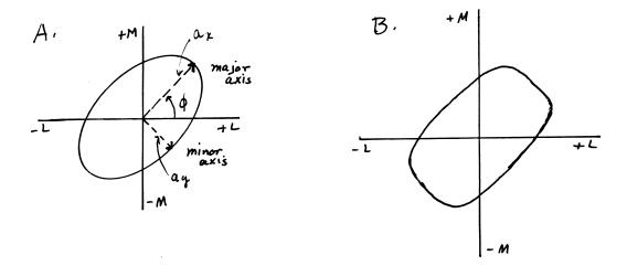
Figure 12.6: Detection contours predicted from (A) an ellipse and (B) a superellipse with an exponent of about 4.
