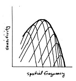
Figure 15.1: A schematic multiple channel model. The figure shows eight different channels, each rather narrowly tuned to a different range of spatial frequencies. The heavy line shows the the overall CSF. Each of the eight channels has been shifted vertically to model the overall CSF as the upper envelope of the channels.
