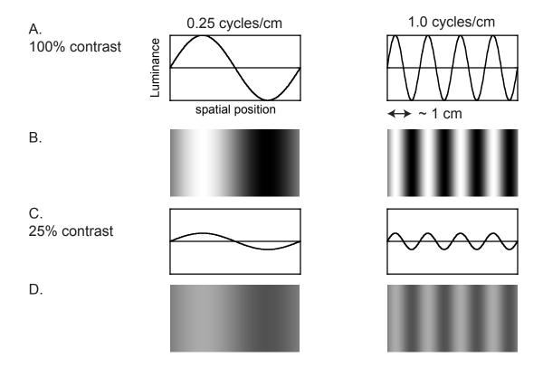
Figure 5.2: Sinusoidal gratings: variations of spatial frequency and contrast. A. Graphs of the variation of luminance with spatial position across the video screen, for sinusoidal gratings of two different spatial frequencies: 0.25 and 1.0 cy/cm, all at 100% contrast. B. Simulations of how these two sinusoidal gratings would appear. C. Graphs of the same two gratings at 25% contrast. D. Simulations of the appearance of these two 25% contrast gratings.
