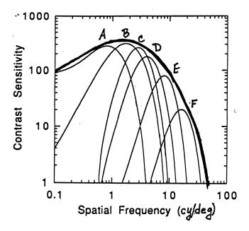
Figure 15.7: Wilson and Gelb's six-channel model. The figure shows the six channels of the model, labeled A through F. The heavy line shows the overall CSF that would be predicted from these channels set to these sensitivities. [Modified from Banks and Crowell (1993).]
