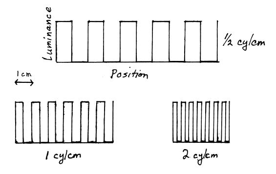
Figure 4.1: Physical specification of a square wave grating. The sketches show variations in luminance across spatial position. One cycle of a grating consists of one high-luminance and one low-luminance region. The spatial frequency of each grating is specified by the number of cycles per centimeter (cy/cm).
