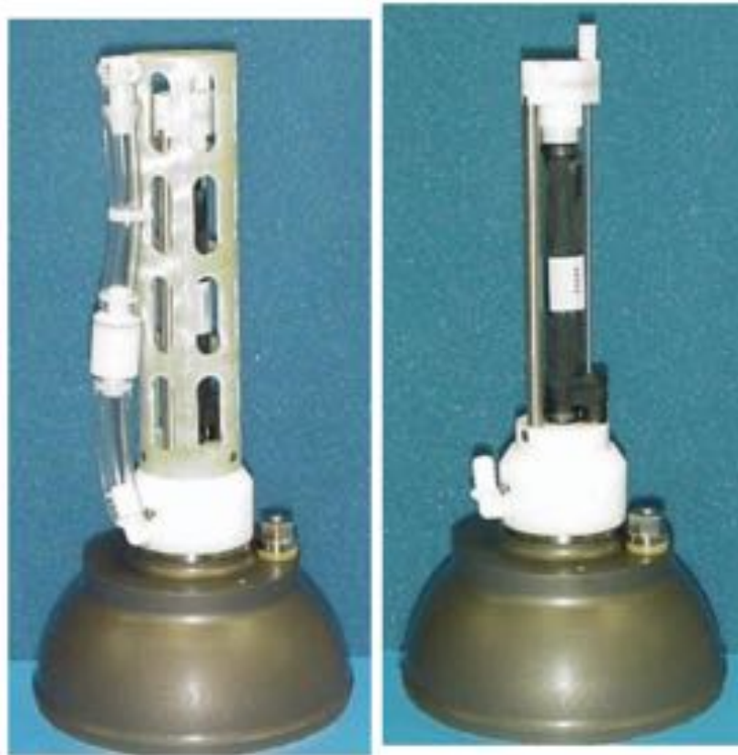
Photo B: Module with guard removed to show conductivity cell
