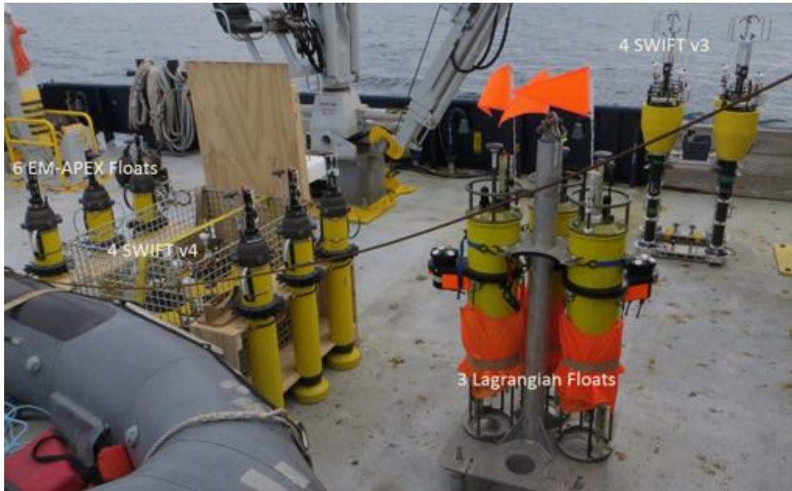
Figure 2.1: MLFs, EM-APEXs, and SWIFTs on deck of R/V Sproul.
