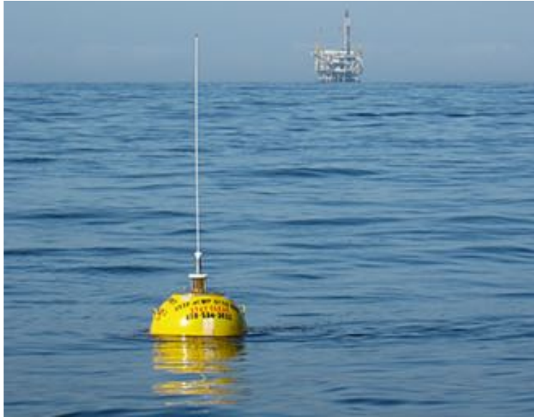
Figure 3.2: A Datawell Waverider from the CDIP wave buoys. Source: cdip.ucsd.edu/
