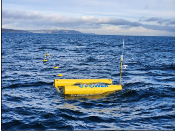
Fig. 1. Tiger Ray Wave Energy Converter and four tethered SWIFT buoys.
