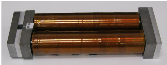
FIGURE 3. GEN 0 MAGNETOSTRICTIVE GENERATORS WITHOUT COMPRESSION HARDWARE (13.3 cm W x 5.7 cm D x 37.5 cm L)
