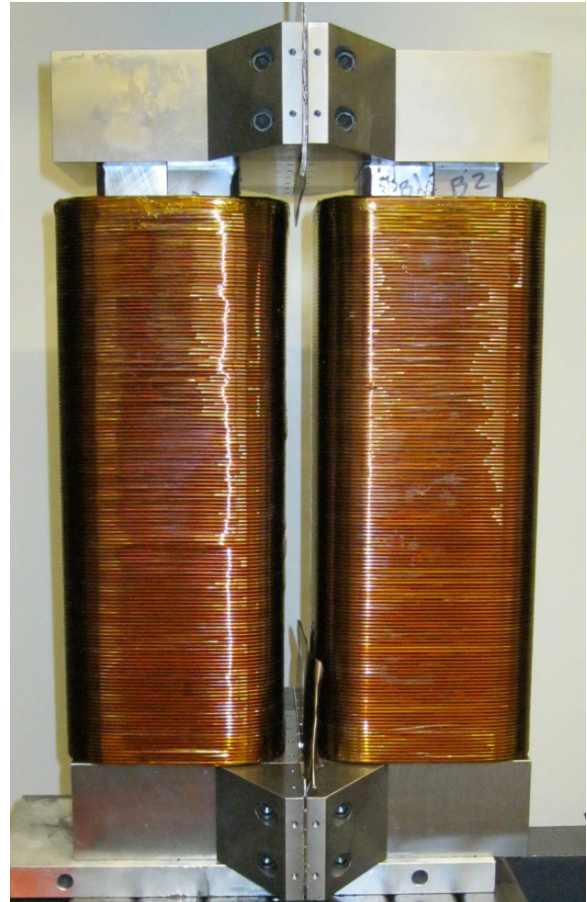
FIGURE 6. “GEN 2” MAGNETOSTRICTIVE GENERATOR (34.6 cm W x 31.8 cm D x 58.42 cm L)
