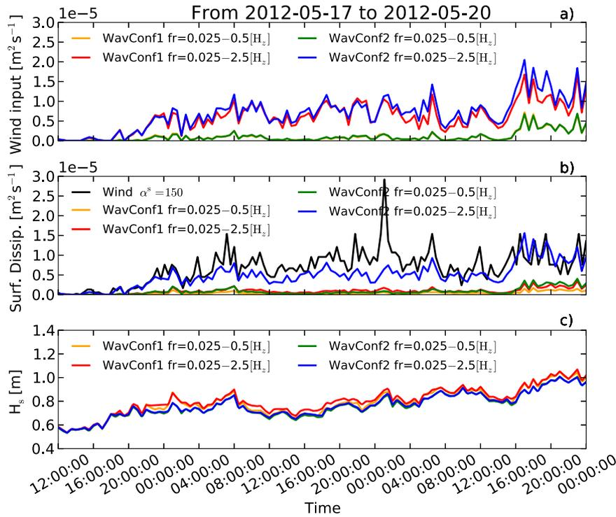
**Fig. 13.** Time series of wave model wind input source term (a), wave model surface dissipation sink term (b) and significant wave height (c). The black line in the bottom panel is calculated for equivalent surface dissipation based on surface flux of TKE from surface shear velocity cubed ( $S_k^{ds} = F_k^s = \alpha^s u_*^3$  for  $\alpha^s = 150$ ).
