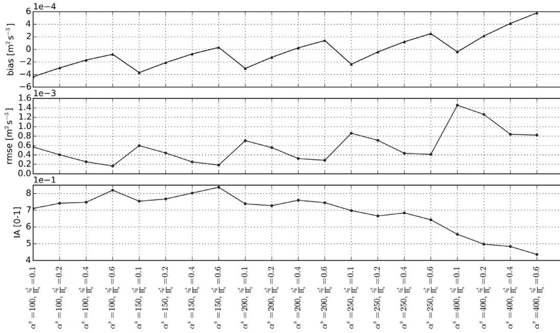
Fig. A.1. Sensitivity analysis experiment for investigating the effects of the surface roughness ( $z_0^s$ ) and  $\alpha^s$  on turbulence dissipation rate modeling results.
