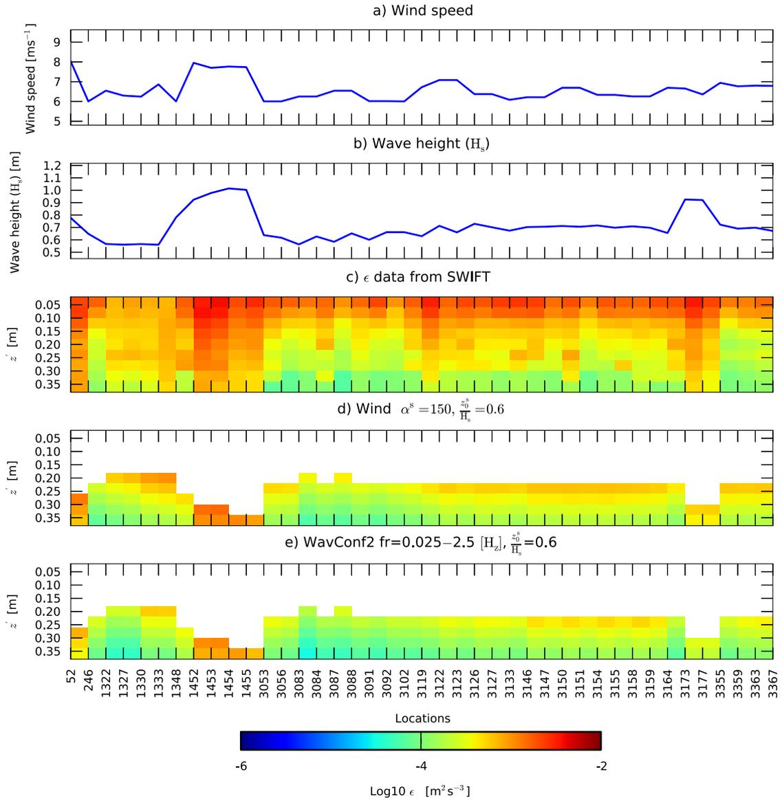
**Fig. 9.** Comparison of measured and modeled turbulence dissipation rate ( $\epsilon$ ) for all SWIFT locations. (a) Wind speed, (b) significant wave height, (c) SWIFT measurements, (d) modeled with TKE injection by surface wind friction velocity cubed with  $\alpha^s = 150$  and  $\frac{z_0^s}{H_s} = 0.6$  and (e) modeled with TKE injection by wave model surface dissipation of Wavconf2 with  $fr = 0.025-2.5$  [Hz],  $\frac{z_0^s}{H_s} = 0.6$ .
