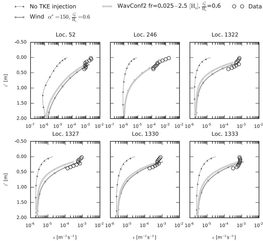
**Fig. 6.** Profiles of the turbulence dissipation rate ( $\epsilon$ ) at the top 2 [m] of the water column. The comparison made for three different TKE surface flux boundary condition results from a  $k-\omega$  two equation turbulence closure model and the measured quantity from 5 min bursts averaged SWIFT observations. The observation locations are shown in Fig. 3 by 6 black rectangles.
