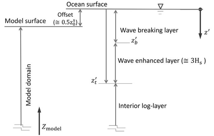
**Fig. 1.** Simplified schematic description of water column surface layers affected by breaking waves. Here  $H_s$  and  $z_0^s$  are the significant wave height and the surface roughness (see Section 2.2.1).
