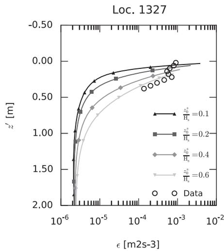
**Fig. 7.** Sensitivity of the turbulence dissipation rate ( $\epsilon$ ) profiles to the choice of  $z_0^s$ . The comparison made for four different surface roughness of  $\frac{z_0^s}{H_s} = 0.1, 0.2, 0.3$  and  $0.4$  at location 1327. See description of Fig. 6.
