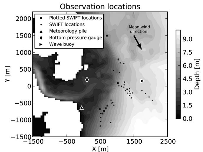
**Fig. 3.** Observation locations at New River Inlet. Circles and rectangles are SWIFT locations ( $N = 41$ ). Diamond is the location of bottom mounted pressure gauge. The up- and right-triangles are the locations of the meteorological pile and wave buoys.
