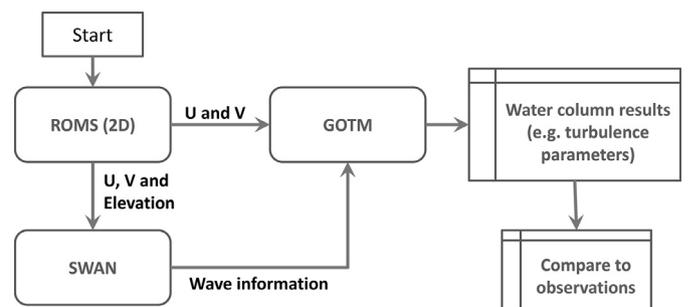
**Fig. 4.** The flowchart of coupling algorithm among models. ROMS (2D) and SWAN models run for the whole domain and time period. GOTM model was executed for each SWIFT observation location separately using information provided by ROMS(2D) and SWAN.
