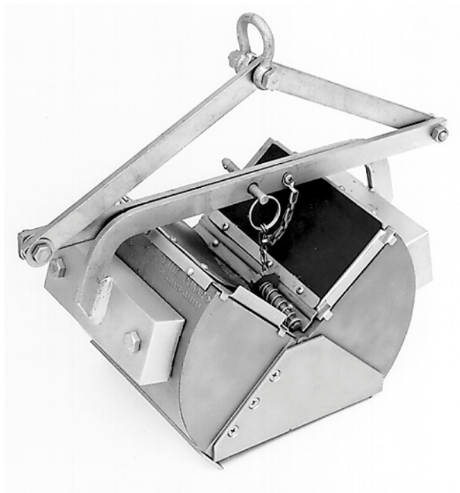
Fig. 4.2 Ponar-type grab samplers (Rickly Hydrological Company 2010).
