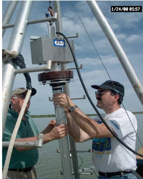
Fig. 4.3 Deployment of 3-inch VibeCore-D Sampler for deep water sediment sampling. VibeCore Brochure 2008.
