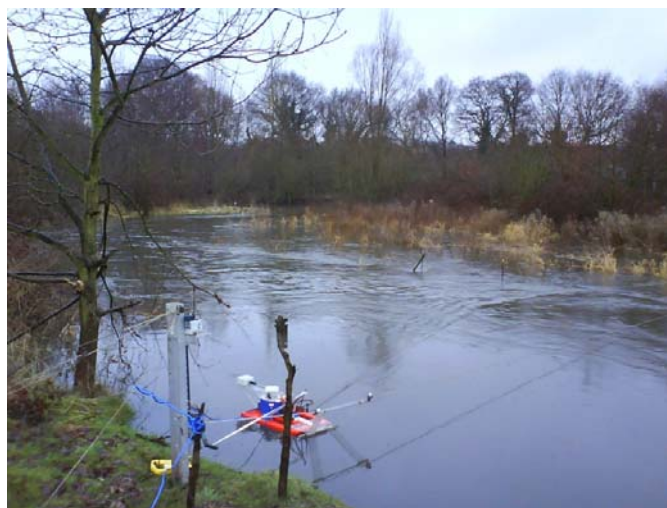
Fig. 4.19 Schematic view of the ADCP cableway system used in Gunawan 2010 (top); The system in use for a measurement in a small river during flood (bottom) (Gunawan et al. 2011b).
