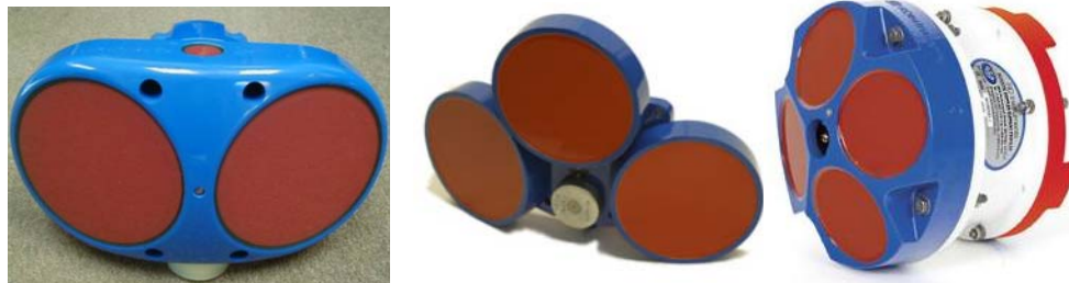
Fig. 4.10 Different types of ADCP beam configurations (RDI 2011)
