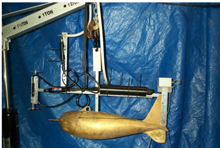
Fig. 4.16 Cable-deployed ADV (CDADV) with sounding weight (Photograph courtesy of Bob Holmes, USGS, 2010).
