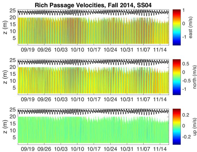
Figure 7: Time series of free-surface and velocity profiles observed at SS04.
