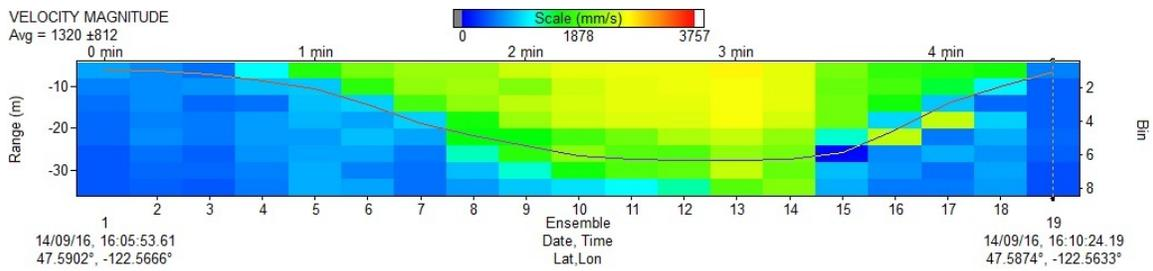
Figure 4: Velocity magnitude along a cross-channel section of Rich Passage from vessel-mounted, downward-looking ADCP measurements.
