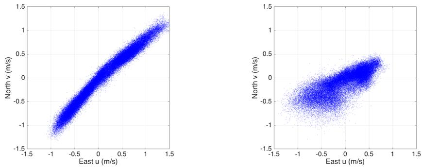
Figure 8: Velocity component measurements about 10 m above the sea bottom at SS02 and SS04.
