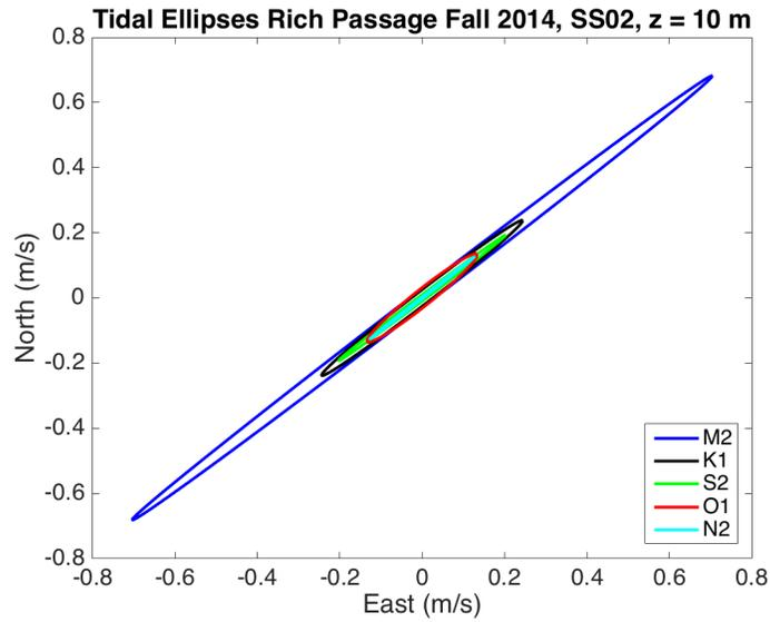
Figure 9: Tidal constituents ellipses for currents measured 10 m above the sea bottom at SS02.
