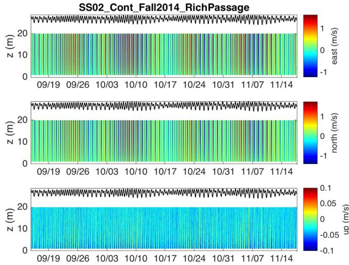
Figure 6: Time series of free-surface and velocity profiles observed at SS02.
