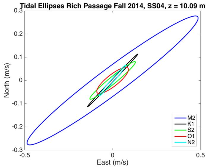
Figure 10: Tidal constituents ellipses for currents measured about 10 m above the sea bottom at SS04.
