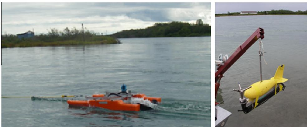
**Fig. 3.** Doppcat platform for down looking Nortek Aquadopp velocity profiler (left) and sounding weight platform for Nortek Vector velocimeter (right) at Igiugig, AK.
