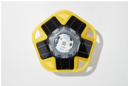
Fig. 1. Free-drifting Spotter configuration. Handles along the hull edge and light, compact structure maximize the device's ease of deployment.
