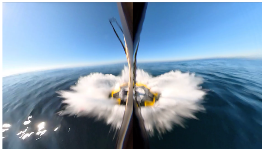
Fig. 3. 360 GoPro screen capture of one of the airdropped Spotters impacting the ocean surface. The GoPro mounting appeared to stabilize the fall, causing this particular unit to land upright and subsequently suffer minimal damage. Units that landed with other orientations experienced higher failure rates.
