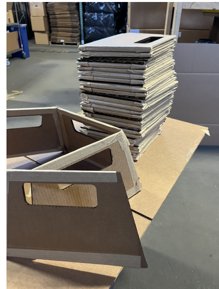
Fig. 4. Cardboard stabilizers to be attached to the air-deployable Spotters.
