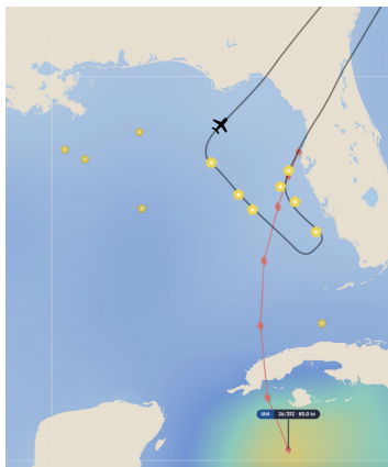
Fig. 8. The locations of air-dropped Spotters are indicated by the larger, yellow pentagons along the black line, which represents the flight path of the aerial deployment platform. The light red line indicates the predicted path of Hurricane Ian's eye close to the time of the deployment - 12:00Z on September 26th, 2022. Smaller yellow pentagons indicate Spotters that had been preemptively deployed by vessels earlier in 2022.
