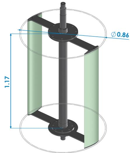
Fig. 1. Rendering of field-scale cross-flow turbine with dimensions in meters.
