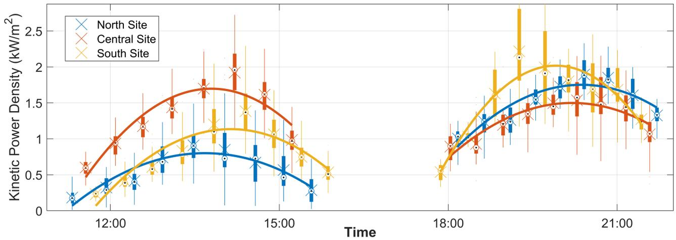
Fig. 4. Boxplots of kinetic power density at candidate sites during ebb (left) and flood (right) tides.
