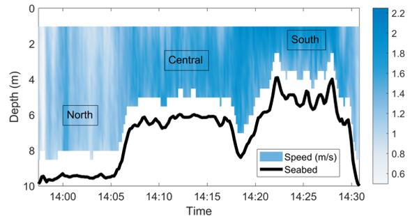
Fig. 6. Typical ADCP bottom track with velocity profile.
