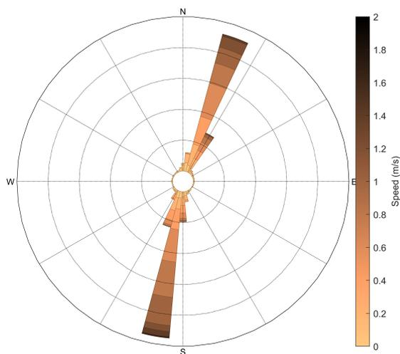
Fig. 8. Flow speed and direction at Central site from bottom-mounted ADCP.
