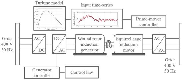
Fig. 4. Schematic of Conn emulator layout
