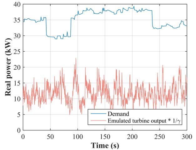
Fig. 13. Grid demand and emulated turbine output
