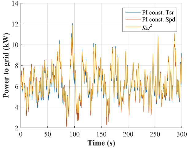
Fig. 9. Real power delivered to grid with 1 s moving average smoothing
