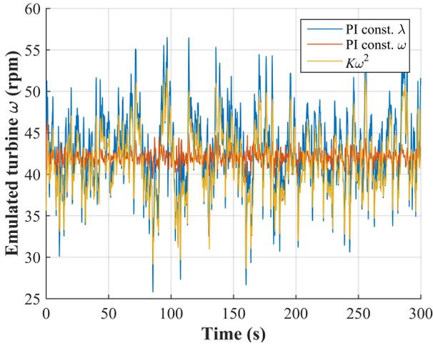
Fig. 7. Emulated turbine speed under control action
