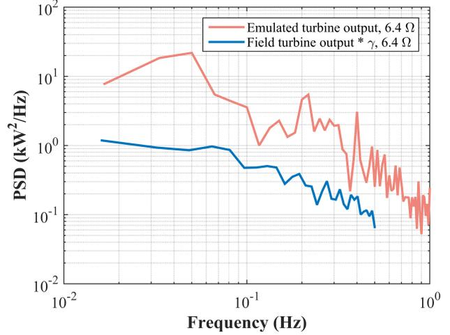
Fig. 11. Dynamic performance comparison between field-tested and emulated real power output
