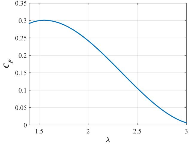
Fig. 3. Estimated performance curve of the RivGen turbine as implemented in emulation assuming a 90%  $\eta_E$
