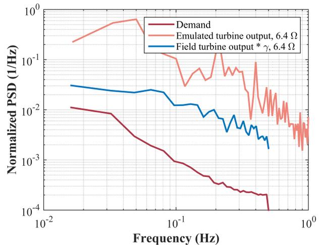
Fig. 14. Grid demand and emulated and field turbine output normalized PSD
