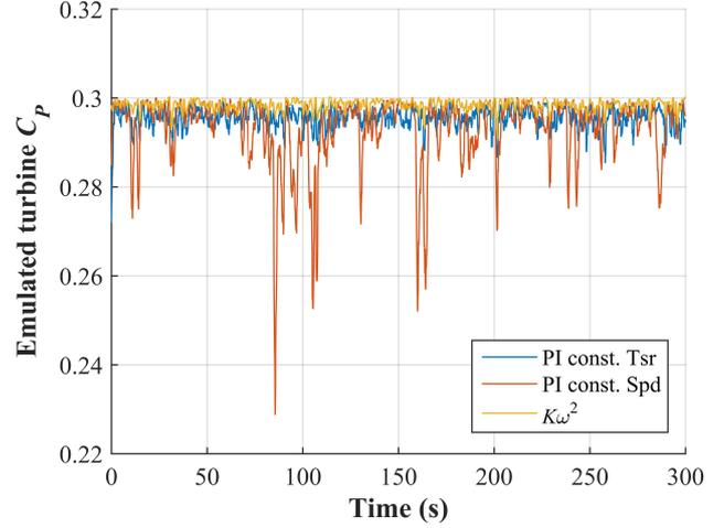
Fig. 8. Instantaneous emulated  $C_P$  with 1 s moving average smoothing
