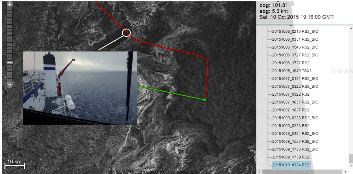
Figure 6. Superimposed RADARSAT-2 image with photo from Sikuliaq on the same day and roughly the same time. Julian day 2015/10/10, 3:34UTC. Photo location: 73.7°, -150.8°. The photo range is approximately 1nm.
