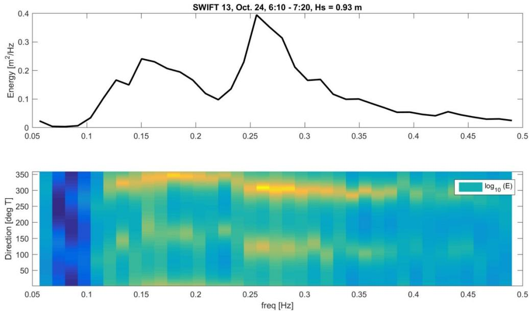
Figure 5. Sample wave energy and directional spectrum.
