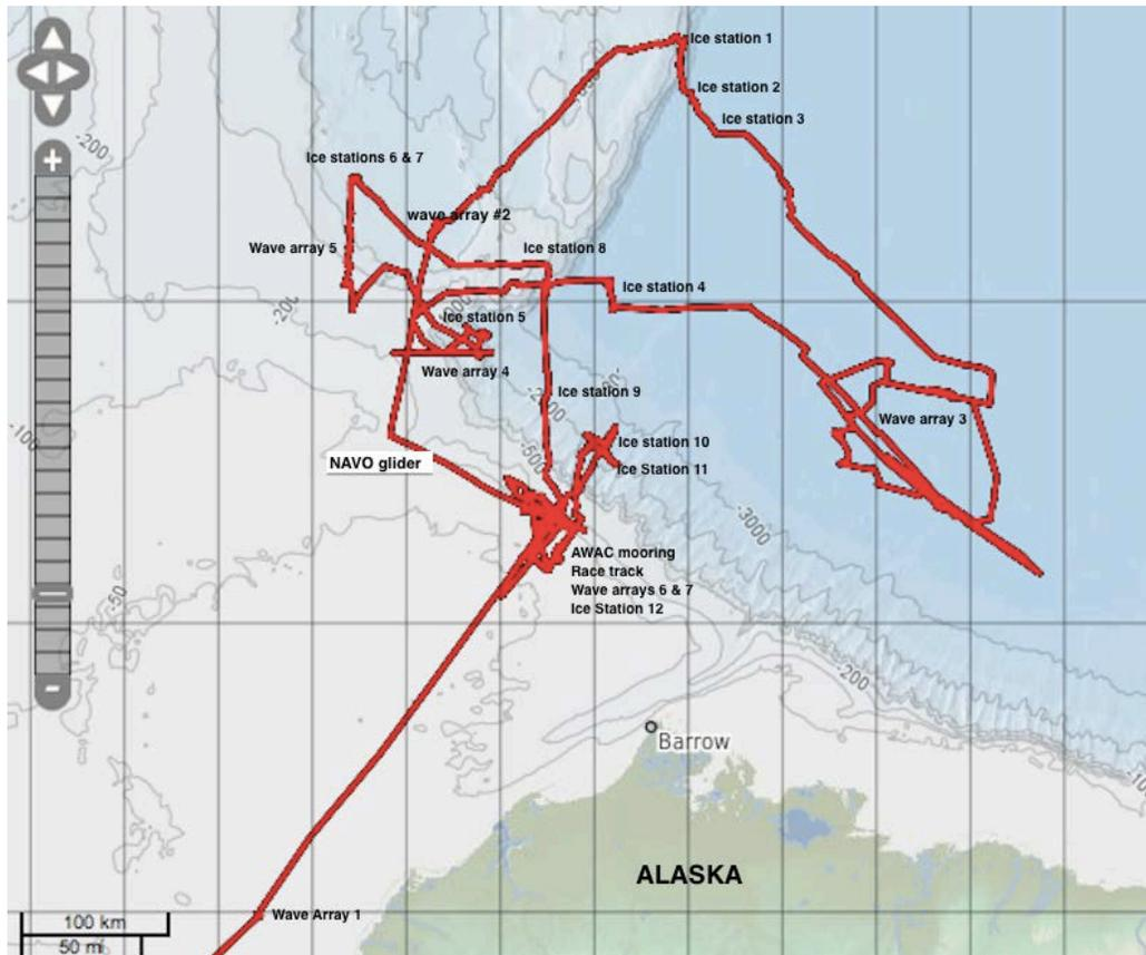
Figure 1. Sikuliaq cruise track. The seven wave tests are shown. Ice stations marked are locations of detailed ice measurements with AUV, LiDAR, and other instruments.
