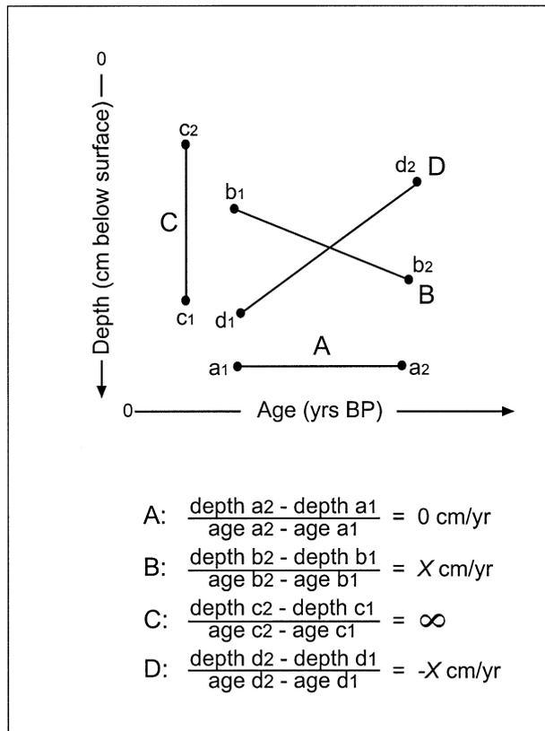
Figure 2. Hypothetical accumulation rates: radiometric age as a function of sample depth. Line A models zero accumulation, Line B models a positive accumulation rate, Line C models an infinite accumulation rate, and Line D models a negative accumulation rate.
