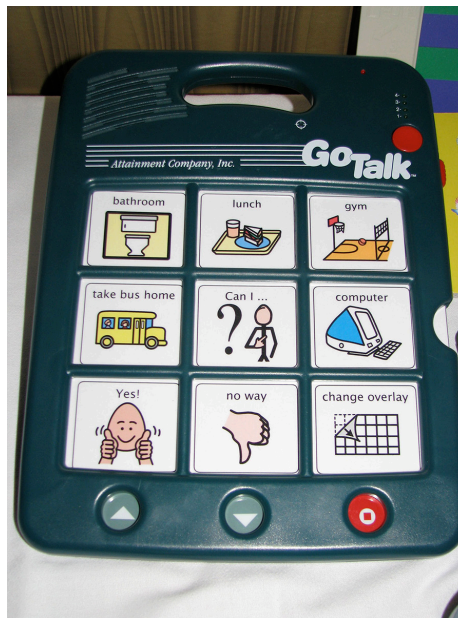
Figure 5.2: The GoTalk is a commonly used speech generation device that predates the use of general purpose mobile devices for similar purposes. Photo credit CC Flickr user bknittle.
