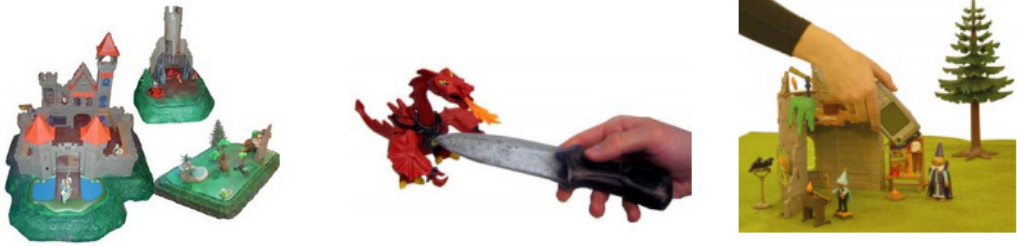
Figure 10.3: Augmented Knight's castle game (Farr et al., 2010) that uses RFID tags and readers to identify when the player interacts with objects.
