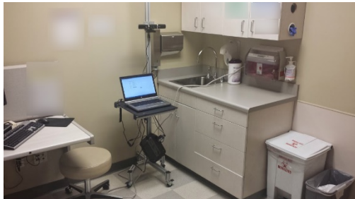
Figure 3. ShoulderCam in a medical exam room. The height of the Kinect sensor is adjustable.
