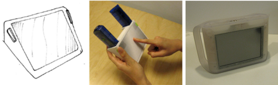
Figure 1: Artifacts from Participant 4 showing the progression of the design from an initial sketch, to a low-fidelity prototype, and then to a functional prototype.
