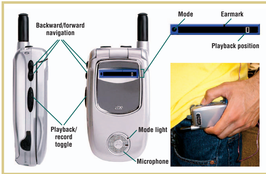
Figure 1. The Personal Audio Loop, which can be attached to a belt clip (inset), has three buttons that control navigation within the recording and record/playback mode. A timeline indicates the current mode and relative place in the buffer.
