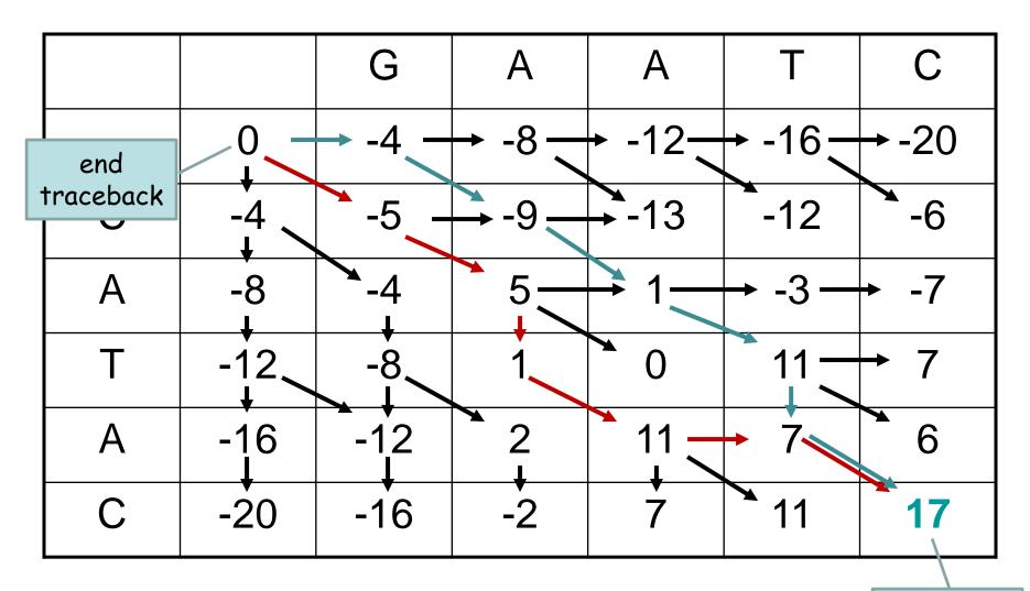
Fill DP matrix from upper left to lower right, trace back alignment from lower right corner.
